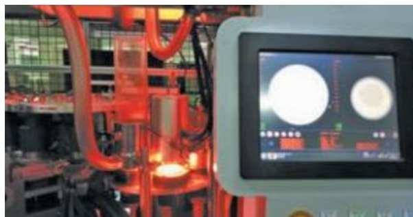
INFRARED RAY AUTOMATIC INSPECTION
